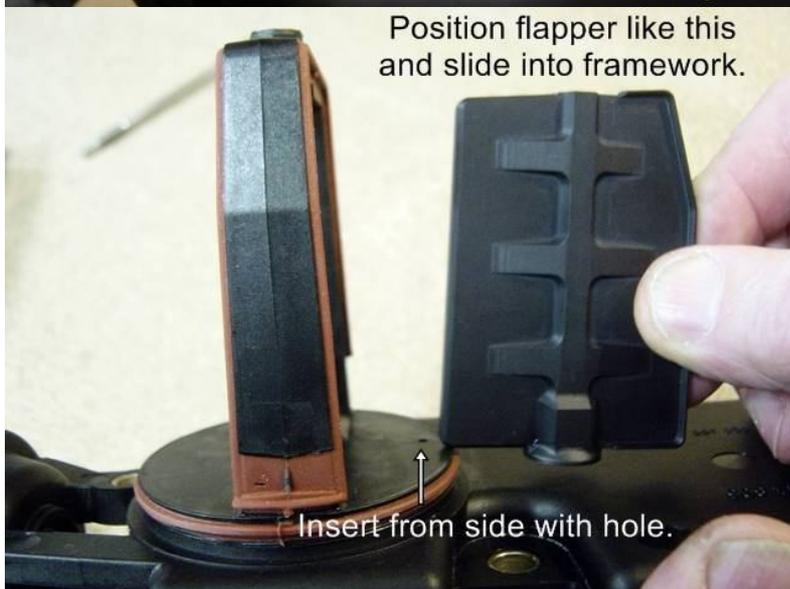
Position flapper like this and slide into framework.
