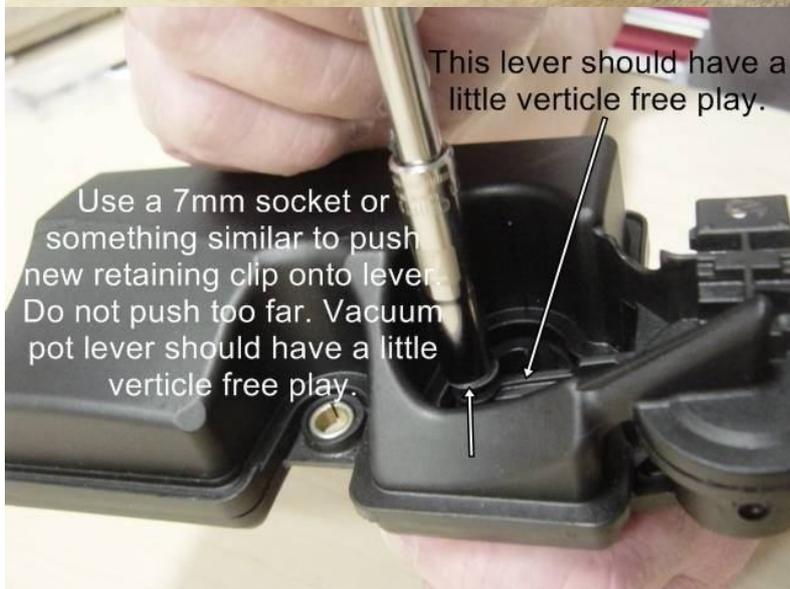
Use a 7mm socket or something similar to push new retaining clip onto lever. Do not push too far. Vacuum pot lever should have a little verticle free play.
