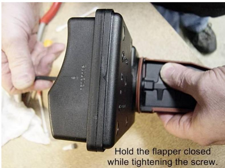
Hold the flapper closed while tightening the screw.
