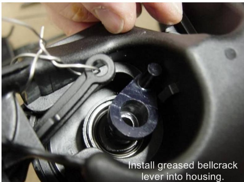
Install greased bellcrank lever into housing.
